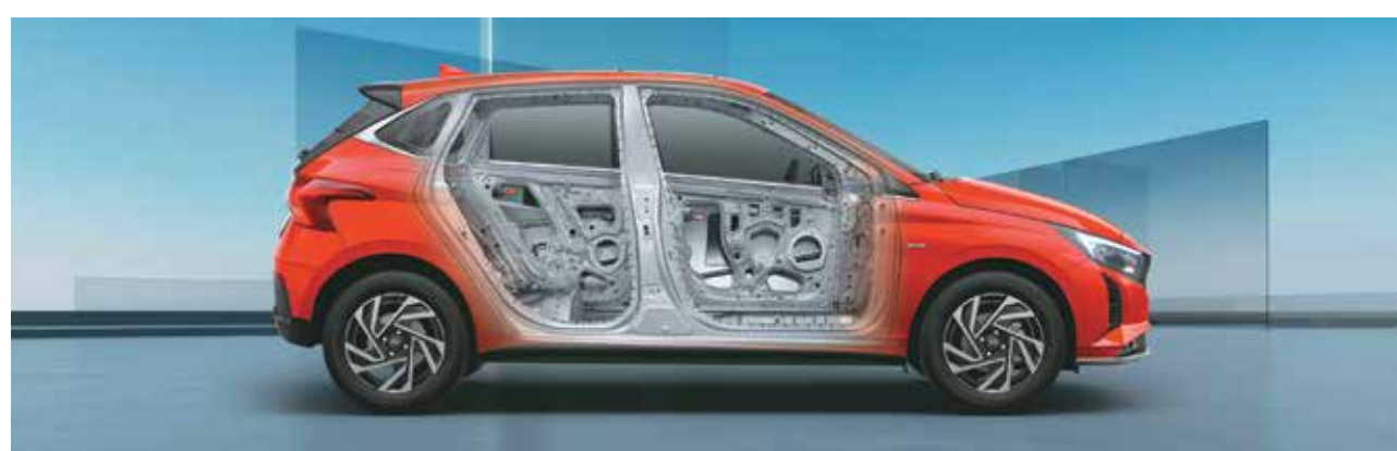
Strong body structure (with AHSS and HSS)
